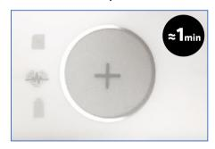
Once the display of the operating is the device state over. begins calibration phase automatically. During the calibration, the LEDs flash white one after the other
