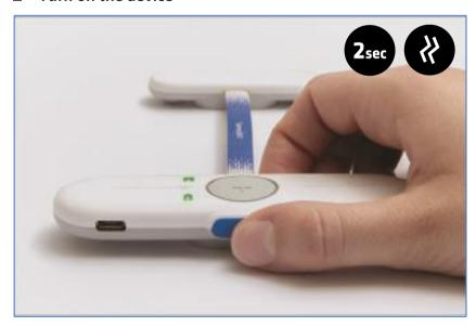
To turn the device on, press the ON/OFF button for 2 seconds. The device briefly vibrates twice and automatically displays the operating state of the device for 5 seconds.
