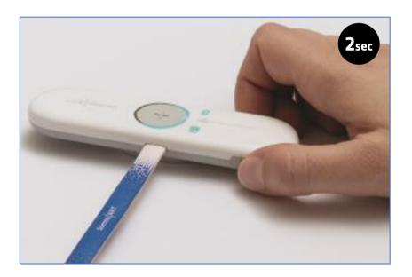
Press the button for 2 seconds to turn on the Bluetooth.
