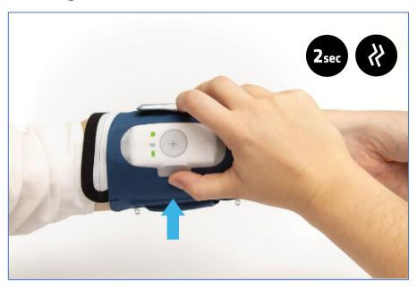
To turn the device on, press the ON/OFF button for 2 seconds. It will briefly vibrate twice and automatically display the operating state of the device for 10 seconds.
