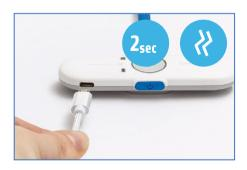
Connect the USB cable to the device then to the computer. The device briefly vibrates twice and automatically displays the operating state of the device.
